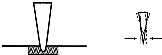
Figure 10. Tip Movement and Sinking. As the tip sinks into the polymer above T_g , the movement at the tip is restricted due to the surrounding polymer. Increased material must be moved by the tip to achieve the same amplitude response
